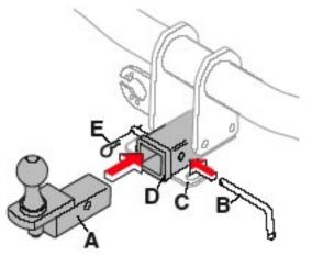
A - ball holder, B - locking bolt, C - safety wire attachment, D- hitch assembly, E - cotter pin
